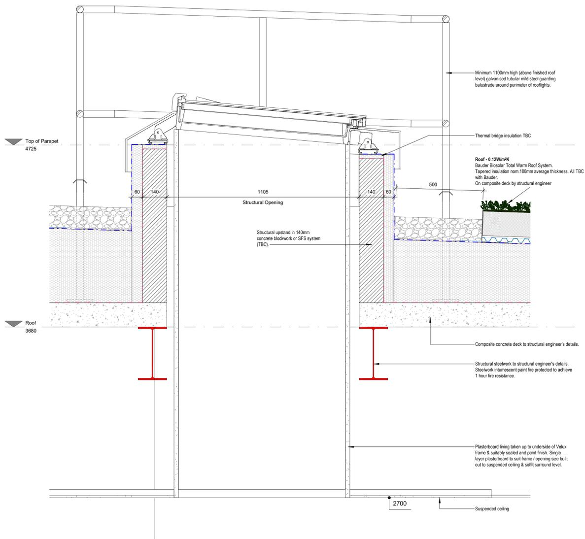
**2** | Rooflight Cross Section
