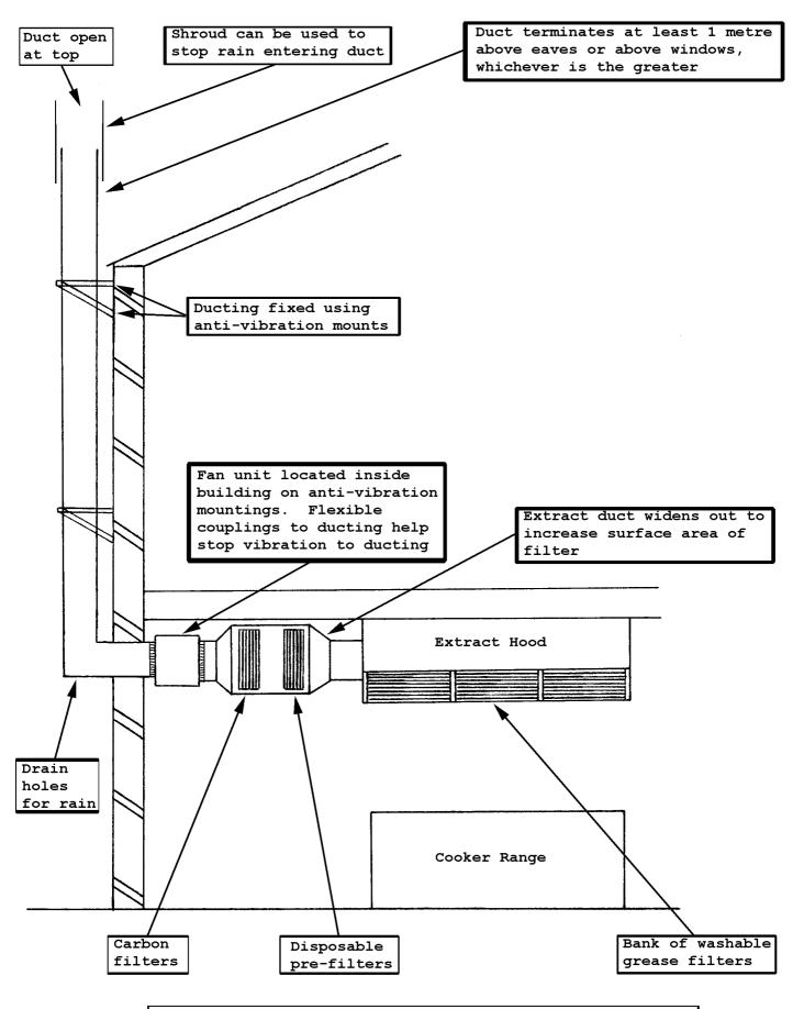
All filter units must be easily accessible for maintenance
