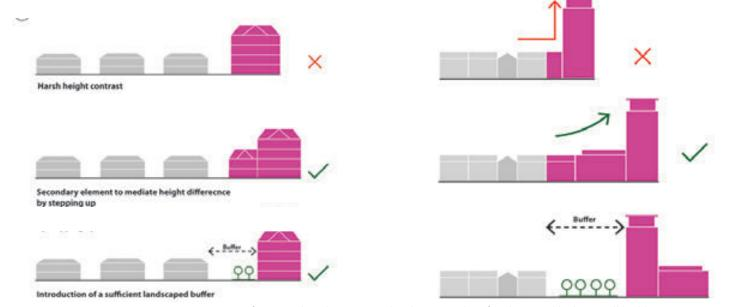
Figure f.13: Avoid stark contrast in height - examples of mid-rise and high rise tall buildings
