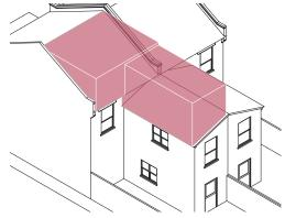
Figure i.37: L outrigger roof extensions will be refused as they become overbearing and can cause loss of daylight to neighbouring properties, as well as loss of the original pitch of the property's roof.
