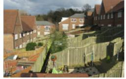
Image f.43: Additional care needs to be taken to accommodate awkward slopes. In this example inadequate consideration has been given to the configuration of the front threshold and the back gardens.
