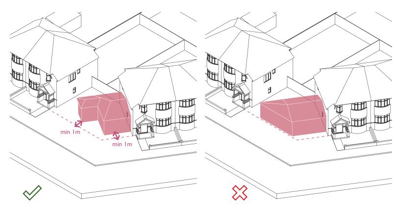
Figure i.41: Corner plot extensions should be staggered parallel to the main house and set back Im from the property boundary.
